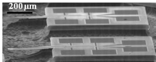
Figure: Scanning electron microscopy picture of micro-devices based on functional oxide thin films
